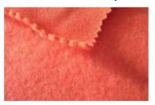
Fleece is a type of weft insertion jersey. Weft insertion fabrics are weft knitted fabrics in which an additional yarn is inserted for each course. These additional yarns are not knit, rather they are held by the loops in each course of the fabric.
