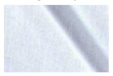
These are primarily used for bed coverings. They are medium weight, closely woven fabrics woven either in plain or twin weave. Sheeting fabrics are made in different widths. High-quality cotton sheeting's are made in plain weave with a width of 64" x 58" and in a twill weave with a width of 60"x72".
