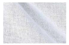
It is a stiff coated fabric made from a lightweight loosely woven fabric, impregnated with adhesives and fillers. This fabric is used as interfacing to provide support and shape retention to necklines, collars, belts, cuffs, waistbands, button closures etc. in garments. They are also used as reinforcements for handbags and other articles.
