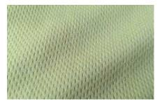
Bird's eye is a double-knit fabric with a combination of tuck stitches along with knitting stitches. The tuck stitch creates interesting eyelet or hole effect on the fabric surface resembling a bird's eye. Fab. The fabric usually made of multicolored threads creating scrambling effect. The fabric may be made with designs having eyelets. They are a popular clothing fabric, especially women's wear.
