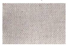
Fustian is a heavyweight fabric made with a linen warp and cotton wefts or fillings. The Fustian fabrics are usually used for menswear and the name "Fustian" is generally used to denote heavy fabrics in the past.
