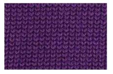
Flat or Jersey Knit fabrics have visible flat vertical lines on the front and dominant horizontal ribs on the back of the fabric. The flat or jersey knit stitch is used frequently, it is fast, inexpensive, and can be varied to produce fancy patterned fabrics. A major disadvantage of regular flat knits is their tendency to "run" if a yarn is broken. The flat or jersey stitch can be varied by using
