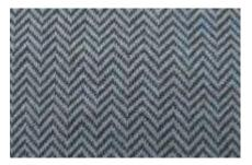
Jacquard Jerseys are single jersey fabrics made of Circular Knitting machines using Jacquard mechanism. They are the simplest method of making patterned fabrics. They are produced with interesting patterns, which may have any of the following:
