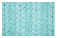
Cable fabric is a double-knit fabric made by the special loop transfer technique. The wales in the fabric have a rope-like an appearance, where plaits are based on the transfer of loops with adjacent wales. The fabric has an interesting surface texture like braids as the loops cross each other. It is widely used as sweater fabric.
