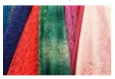
Chiffon basically refers to a light plain weaved sheer fabric with a soft drape of alternate Sand Z-twist crepe yarns. The twist in the crepe yarns puckers the fabric slightly in both directions after weaving, giving it, some stretch and a slightly rough feel. These fabrics when held up to the light, strongly resembles closely woven netting.
