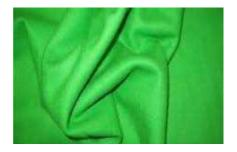
Baize is a smooth, dense, durable textile fabric made from wool and cotton blends generally used on gaming tables such as snooker tables, billiards tables, and blackjack tables. The durability and smooth finishing combined with less friction make Baize Fabric a perfect candidate for the surface of the gaming pool tables.
