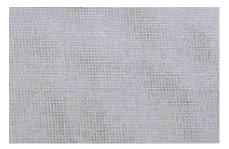
Gauze is plain weave fabrics constructed with more spaces between the threads than regular fabric. Gauze fabric is usually made of cotton, rayon or their blends of soft texture spun yarns.
