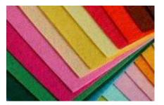
Natural fibers such as wool are pressed and condensed together with heat and pressure to make a sheet of fabrics are called Felt Fabrics. Felt fabrics are non-woven fabrics.
