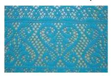
Raschel knits are produced from spun or filament yarns of different weights and types. Most raschel knits can be identified by their intricate designs, the open-space look of crochet or lace, and an almost three-dimensional surface effect design.
