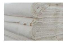
When no finish is applied to the textiles, they are termed as grey fabrics or greige fabrics or unfinished textiles, which of course **does not** refer to the color of the fabric. It implies that no finishing treatment has been given to it. Grey fabrics are used chiefly when the aesthetic values of the end-products are limited.
