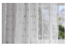
Madras net is used mainly for furnishing such as curtaining. The cloth is an open gauze ground cloth where an extra weft is inserted to produce a motif, this is then woven into the ground cloth. Where there is a surplus floating weft yarn this is then cut away after weaving revealing the motif, the edge of the sheared motif shows shorn ends of a weft yarn.
