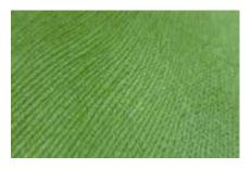
Knitted Velour are Pile jersey fabrics having soft protruding fibers on the fabric surface. Like knit terry, they are also made of an additional set of yarns making pile loops on the fabric surface. However, in Velour, these pile loops are sheared evenly and brushed. It may be dyed and generally available with solid colors. They are used in luxurious apparels like jackets, blouses, dresses etc.
