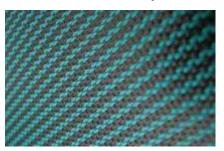
The industrial fabric is a fabric which is usually made from man-made fibers like fiberglass, carbon, and aramid fibers. It covers a wide variety of widths, weights and construction particularly made to meet a specific application. The industrial fabric is used for decorative purposes. The industrial fabric is woven in various thicknesses and constructions in a basic weave, namely plain, leno, satin, basket etc.
