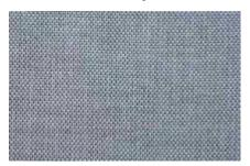
A trade name for a cloth patented in Britain in 1886, which was first manufactured in 1888. The cloth traps air in between its structure, keeping the body cool in summer, and warm in winter. Two threads or ends act as one thread; when a weft thread passes between them, the doup ends twist catching the weft and holding it tightly in place. Very fancy and beautiful clothes can be produced by combining the cross weaving with other weave structures.
