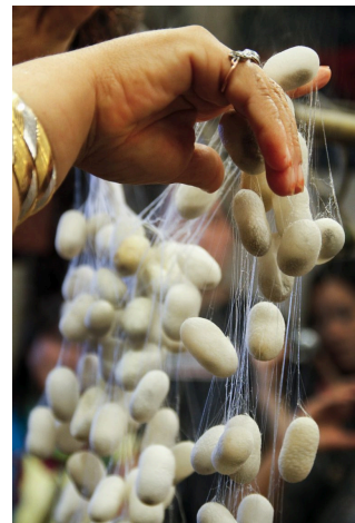
Drawing filaments from cooked cocoons. Image: Pixabay.
