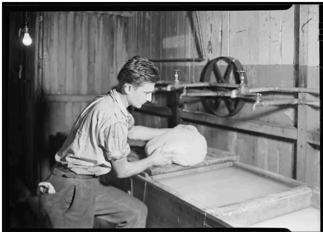
Paterson, New Jersey, 18 March 1937: a rayon skein wrapped in cloth before immersion in solution. Photo: Lewis Hine, US National Archives, via Wikimedia Commons, public domain.
